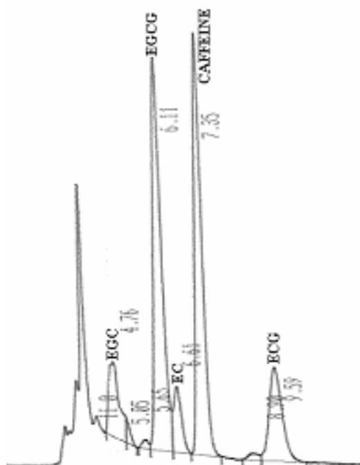
Fig. 2. A typical HPLC chromatogram of green tea extract
