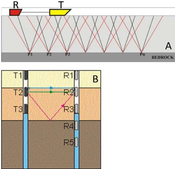
**Figure 1: A) surface multi-fold ground-penetrating radar and B) cross-well tomography ground-penetrating radar data acquisition schemes used in the present work.**
