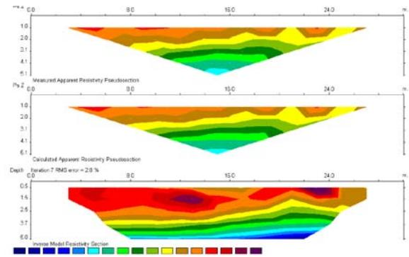
**Figure 5:** Example of 2-D electrical tomography from the area of study: color coded resistivity value (bottom) range from  $1.6 \cdot 10^2$  (blue) to  $2.6 \cdot 10^3$  (dark brown)  $\Omega\text{m}$ .
