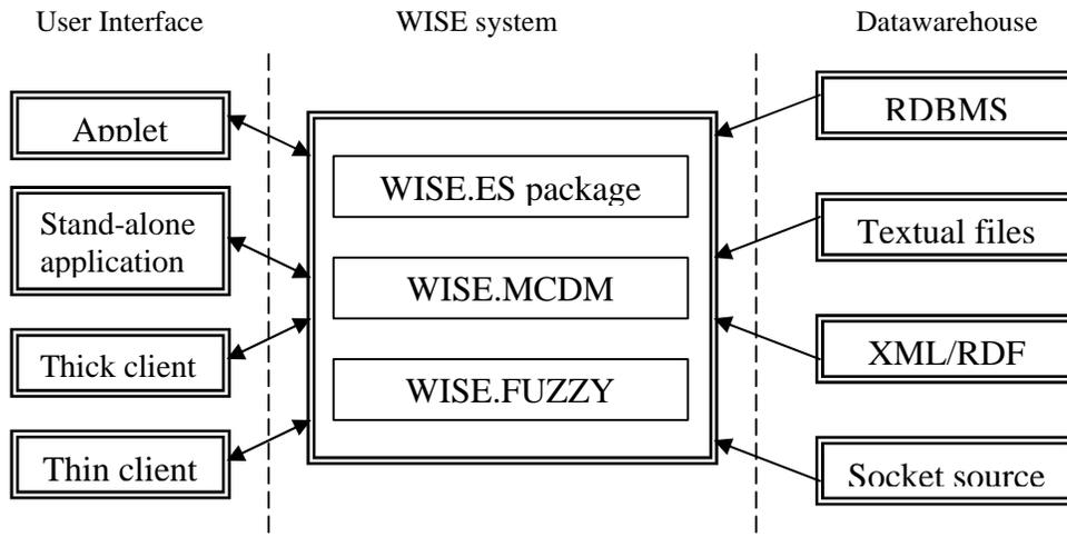
**Fig. 1. WISE based decision support system architecture**
